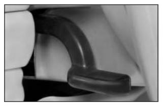
To tilt the wheel, pull down the lever. Then move the wheel to a comfortable position, pull up the lever to lock the wheel in place.
